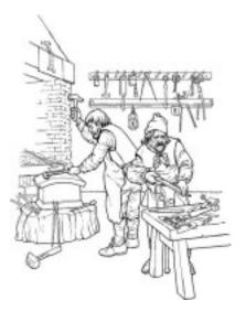
The fireplaces in a blacksmith's shop are called forges. Each forge has a bellows. A bellows is made of leather. It pumps air. The blacksmith pulls a cord to pump air onto the fire. This makes the fire burn hotter.
